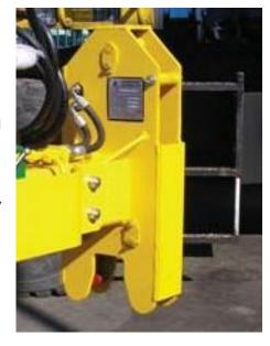
Max. Hyd. Pressure 210 Bar Min. Hyd. Pressure 90 Bar Body Colour 08E51 Yellow Moving Parts Signal Red
