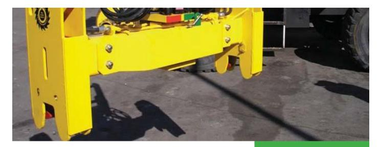
he Thomson RLB20 Rail Beam is the ideal solution for lorry cranes and excavators handling short lengths of new rail or full lengths of scrap rail.
